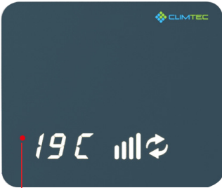
Air temperature sensor (red - air from the street, white - indoors)
